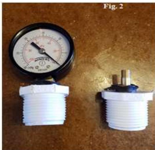
**Figure 2.** Vacuum Gauge and Schrader Valve attached to PVC threaded caps.
