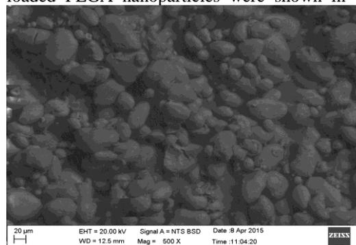
**Fig. 1: Microscopic image of PLGA-Dox under SEM**
