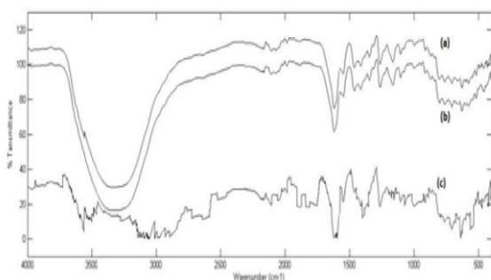
**Fig. 2: FTIR result of PLGA -Dox Nanoparticles: (a) Native PLGA, (b) PLGA -Dox NPs with purification, (c) PLGA-Dox NPs without purification.**
